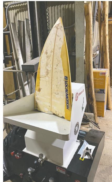
Photo by Tom Loomis The shredder is sized to accommodate surfboards and other items made of thermoset plastics.
